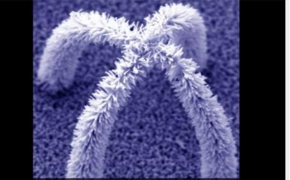
This tiny structure is made up of carbon nanotubes and zinc oxide nanowires grown on a silicon substrate. The photo was taken with a scanning electron microscope.
